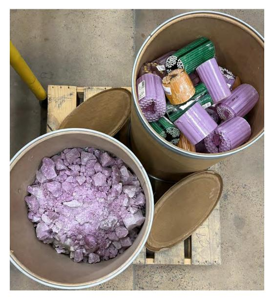
Residual melt material from crystal growth and spent crystal material from fabrication, a waste stream which a team at our SYNOPTICS operation innovated to address.
