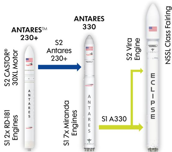
Eclipse is an evolutionary successor to the Antares launch vehicle, offering a significant leap in power, performance, and payload capacity.
