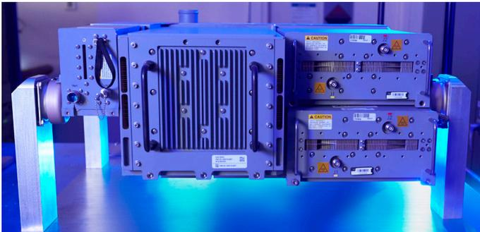
IVEWS incorporates an advanced processor designed specifically for EW applications, and high-powered transmitters. (Northrop Grumman photo)
