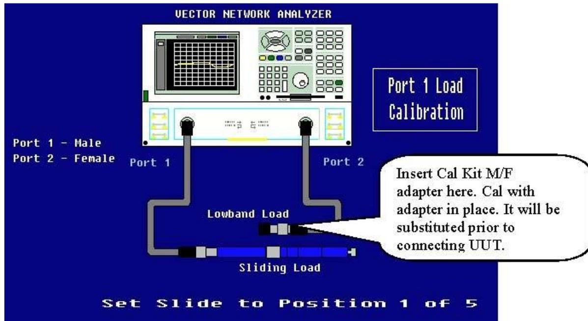
The sliding load calibration is applicable for frequencies above 2GHz.
