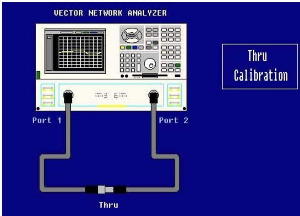
The reference plane length has now been established. Any configuration changes for accommodating connector sexes can only be achieved by substituting equal length adapters.
