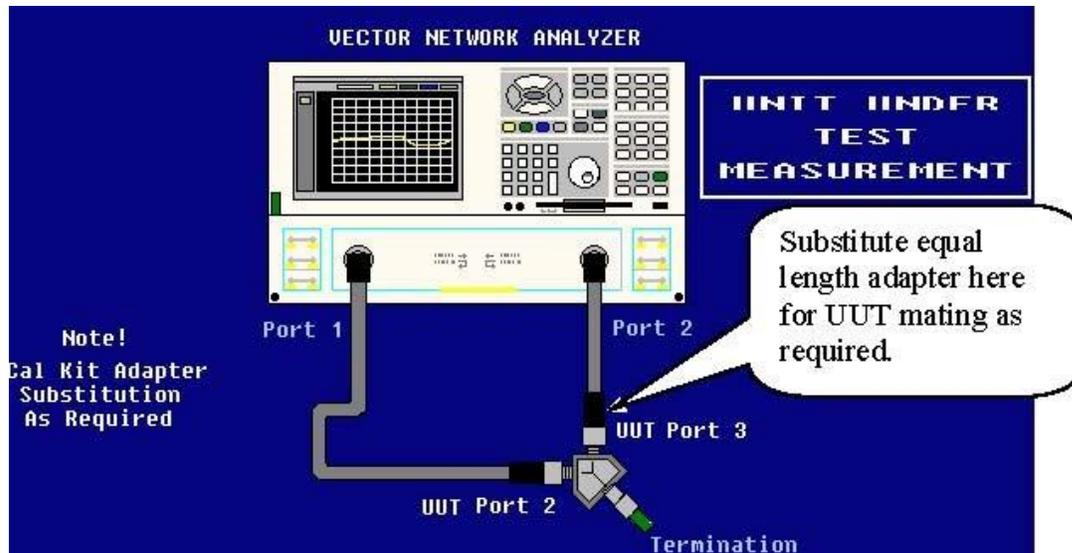
We will need to substitute a male adapter in place of the female adapter used for calibration. The point of the adapter substitution is identified in the graphic below.
