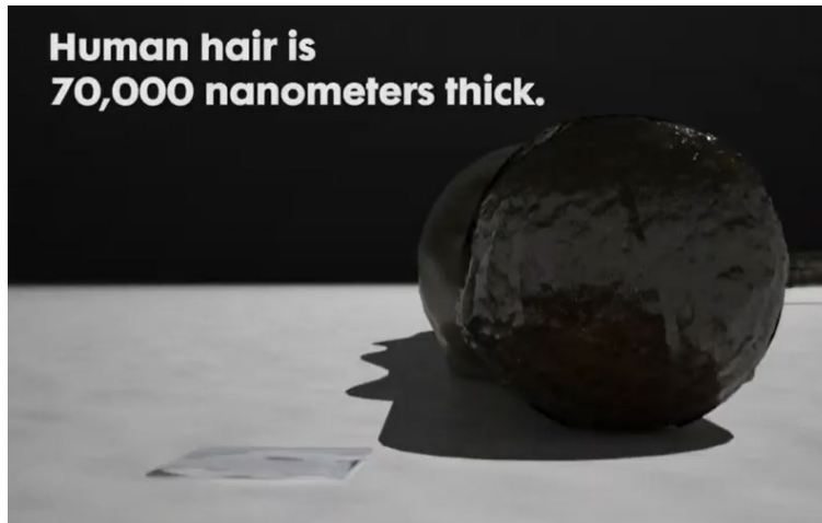
Figure 2-3 – Simulated thickness comparison of human hair with niobium passive film (150 nm thick)
