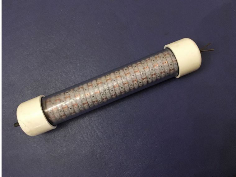
Figure 7-18 - Proxy underwater vehicle with niobium contact and graphite electrode
