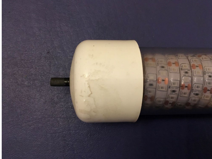
Figure 7-20 - Graphite seawater ground return electrode on back of proxy underwater vehicle
