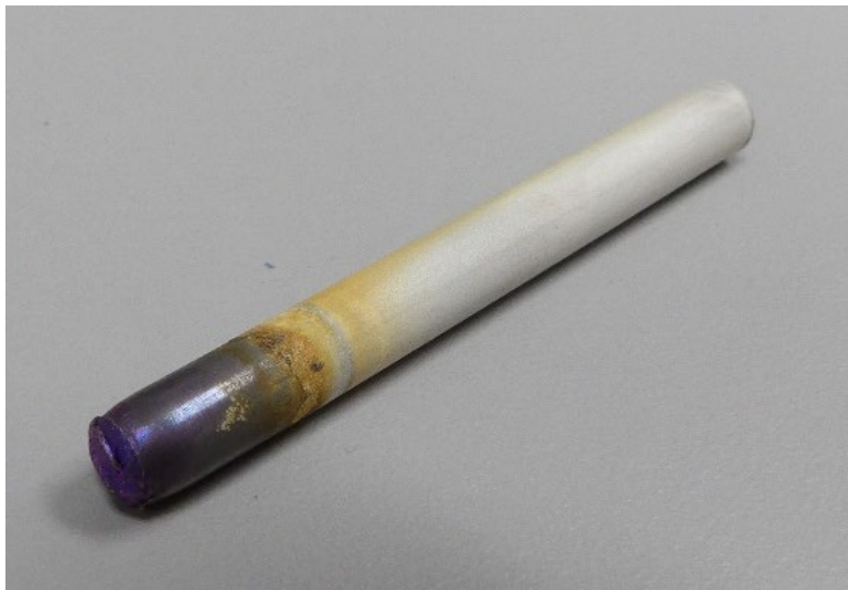
Figure 3-3 - Hard white deposit formed on niobium with an applied voltage of about 100V in artificial seawater
