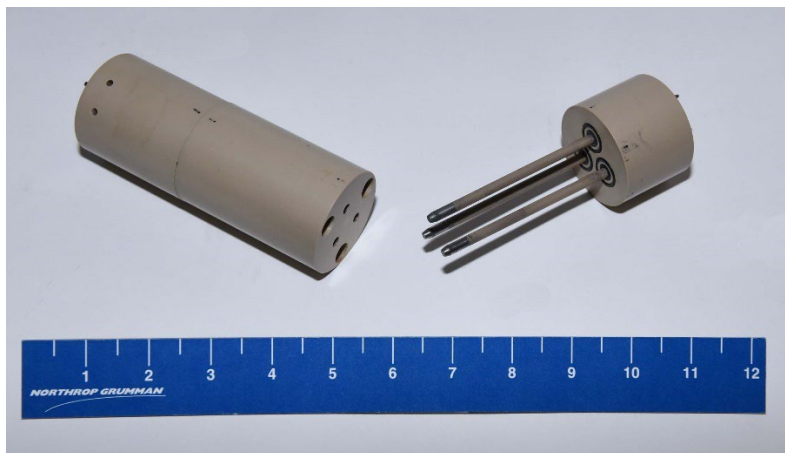
Figure 1-5 - 3-Contact Working Model of the IR Drop Concept
