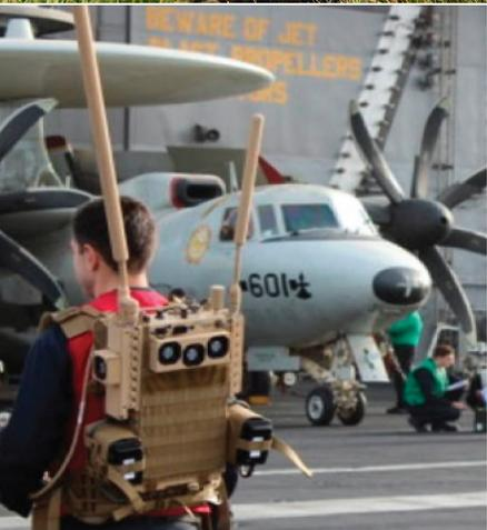
JCREW / DRAKE provides UAS detection (red targets) and performs non-kinetic effects to neutralize drone swarm.
