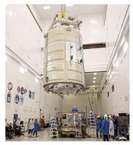
The Cygnus Service Module is mated with the Pressurized Cargo Module at the launch site
