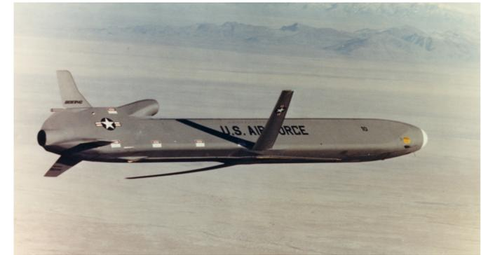
Boeing's AGM-86B ALCM cruise missile flying at a low altitude. Flight altitude is several tens to several hundred meters. (Photo credit: U.S. Air Force)
