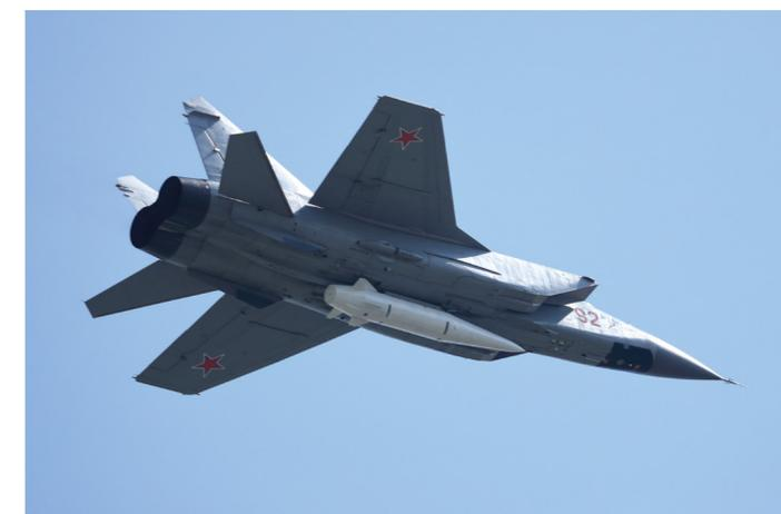
The hypothetical fighter jet and hypersonic weapon in this episode were based on the MiG-31 fighter and Kh-47M2 "Kinzhal," an air-launched hypersonic missile (carried under the fuselage). The missile is estimated to have a scramjet engine and flies more than hundreds of kilometers at hypersonic speed toward its target. (Photo credit: Toshiharu Suzusaki)
