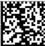
Data Matrix is a two-dimensional barcode that can store from 1 to about 2,000 characters. The symbol is square or rectangular and can range from 0.001 inch per side up to 14 inches per side.
