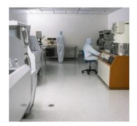
Figure 3. Wafer Processing is completed inside of a class 100 clean room at CEO.
