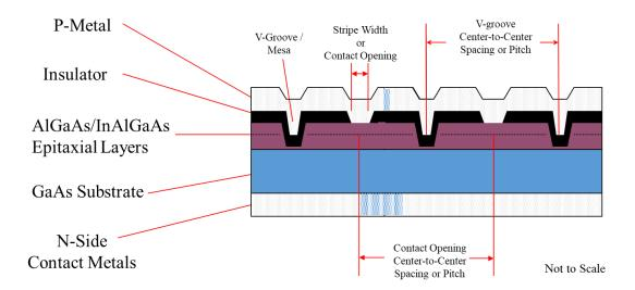
Figure 2. Example cross section of a laser diode device.
