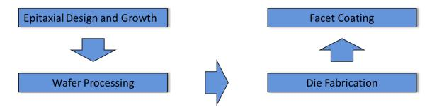
Figure 1. Process flow for the fabrication of high power laser diode devices.
