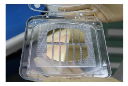
Figure 4. A wafer is shown cleaved into columns. This wafer will later be cleaved into rows forming individual diode bars.
