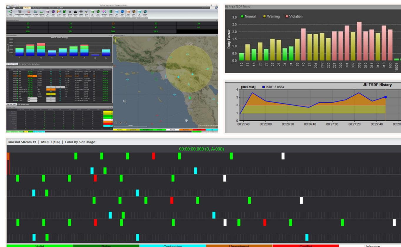
Multiple displays present a seamless tactical picture and summarize multi-TDL network performance. The operator can customize the display to include the most useful data — including signal quality and connectivity information — enabling an at-a-glance view of how networks are performing and which units are experiencing problems.
