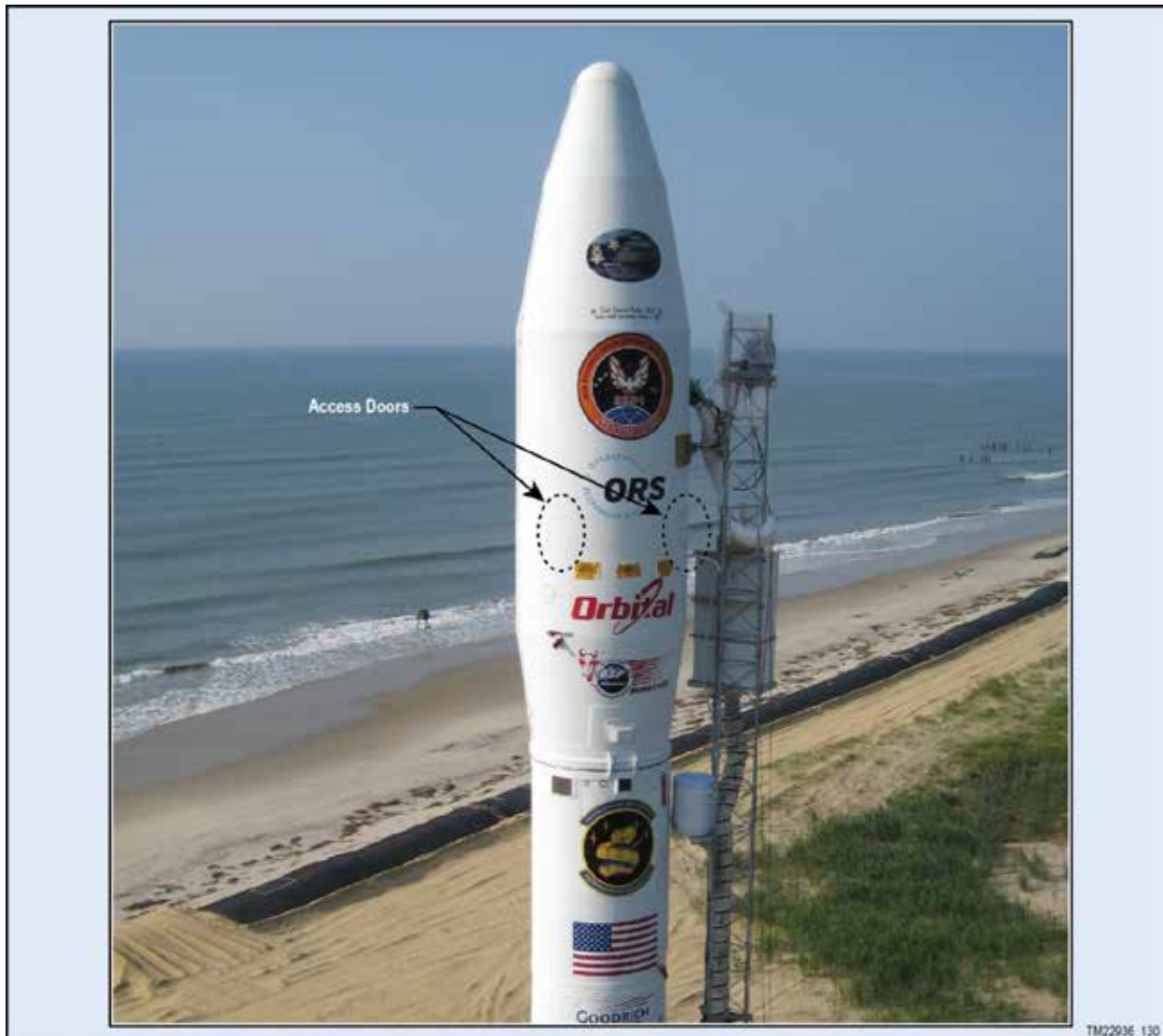
Figure 8.4-1. Multiple Access Doors Were Demonstrated on the Optional Minotaur I Large Fairing
