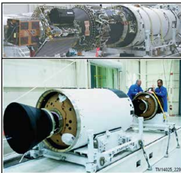
Figure 2.3.2-1. Minotaur I Upper Stack Assembly Processing at Minotaur Processing Facility at VAFB
