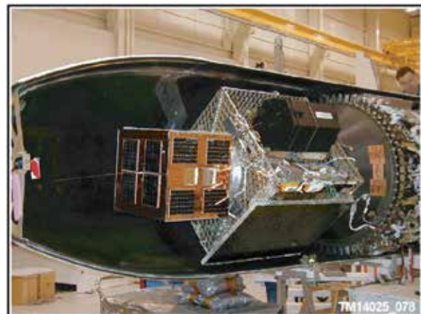
Figure 5.2.4.1.1-2. JAWSAT Multiple Payload Adapter Load Bearing Spacecraft
