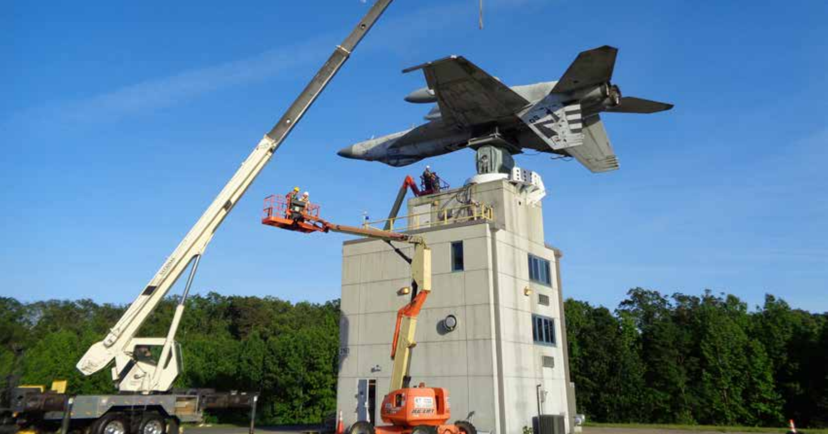
▶ Northrop Grumman's Next Generation Jammer-Low Band demonstration unit for the EA-18G Growler successfully underwent testing at the U.S. Navy's Facility for Antenna and RCS Measurement and Air Combat Environmental Test and Evaluation Facility. Photo source: U.S. Navy
