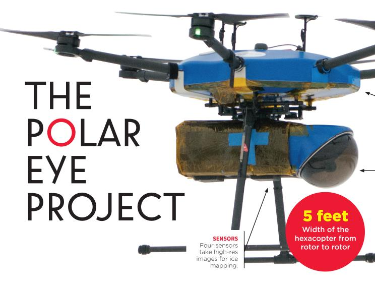
How a team of innovative aerospace engineers tackled a problem here on Earth: Designing a weatherproof drone that can track the loss of Arctic sea ice, which is threatening the lives of polar bears.
