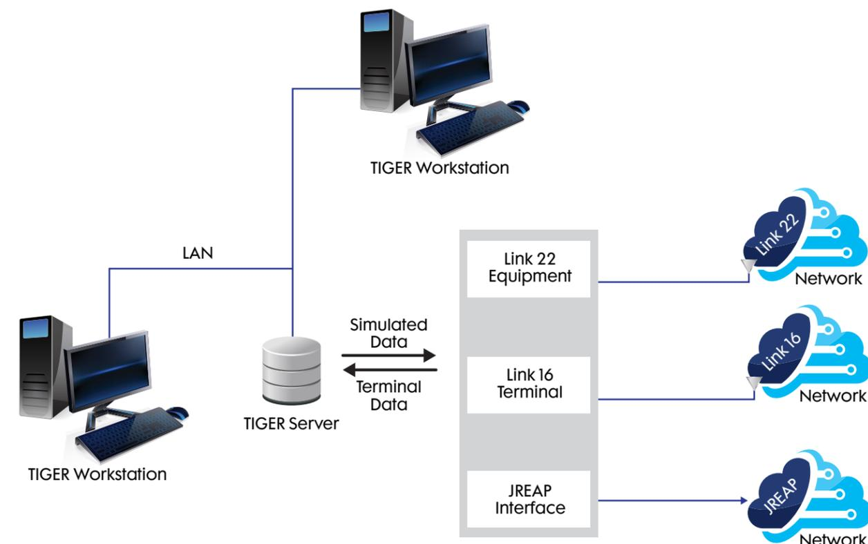
The above configuration can be used to inject simulated data, either ad hoc or via pre-scripted scenarios, from any TIGER workstation to any of the connected test networks. TIGER supports most TDLs, including Link 16/11/22, DIS, JREAP, and SIMPLE. All messages on the test networks, as well as the test Tactical Situation Display, are viewable on any TIGER workstation.
