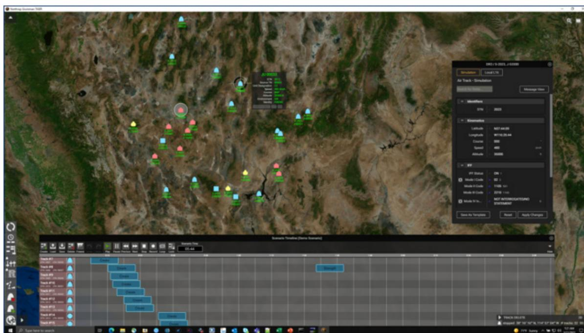
The Tactical Situation Display shows filterable track symbology. During test the user can switch between this window and the Message Monitor. The Message Monitor displays tactical messages, as well as scenario and operator-initiated events, in an organized, user-readable format.
