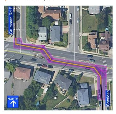
Street closures and vehicle movement during work hours: As we work to complete the piping installation and restoration on Sheridan Avenue, as well as complete the hydraulic pressure test of the full run of piping, 250 feet of Sheridan Avenue north of Laurel remains closed (except to residents who live there), as well as the Central Ave/Sheridan Ave intersection. We want to thank everyone on Sheridan Avenue for moving your vehicles during work hours.
